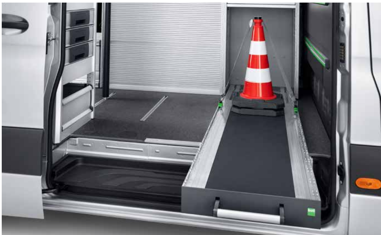
bott vario sliding platform with full extension slide
