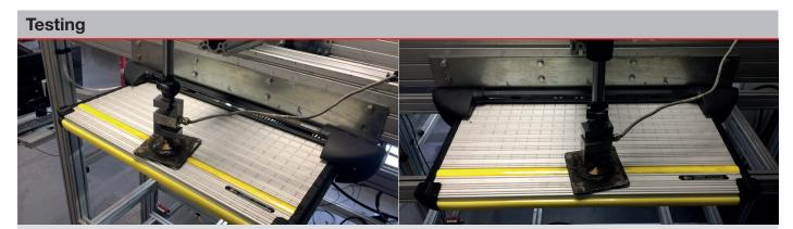
The Glide Step has undergone a rigorous series of tests to ensure safety, reliability and premium performance. This includes cycle load testing, increasing weights in both central and off-centre positions for tens of thousands of cycles.
