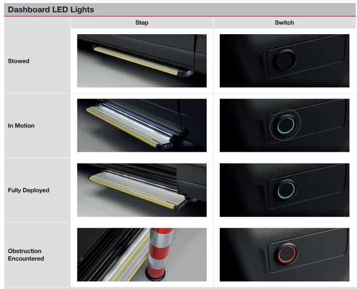
The step is be configured to deploy automatically when the vehicle door is opened and to stow when the door is closed (note: the circular dashboard switch needs to be pressed to power the step).
