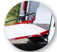
Mobile contact flap to connect to the floor of the van
