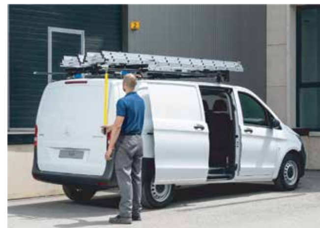
5. The Auto Clamp secures the ladder without additional straps or clamps.
