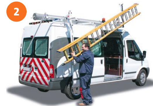
2 - Lift the rear end of the ladder onto the second support;
